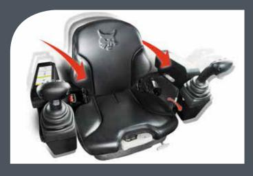
Flexible Joystick positioning: Joystick mounts on our SJC-equipped machines slide forward and backward independent of the seat, adjusting to the individual preference of the operator.
